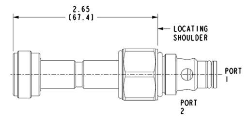
This solenoid-operated, 2-way, 2-position cartridge is a pilot-operated, directional poppet valve. This valve offers 2-position/2-way directional control with a lower pressure drop than its direct-acting counterpart. The valve is available in the normally open and normally closed condition.
