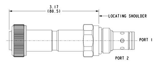
This solenoid-operated, 2-way, 2-position cartridge is a pilot-operated, directional poppet valve. This valve offers 2-position/2-way directional control with a lower pressure drop than its direct-acting counterpart. The valve is available in the normally open and normally closed condition.
