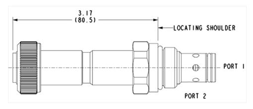
This solenoid-operated, 2-way, 2-position cartridge is a pilot-operated, directional poppet valve. This valve offers 2-position/2-way directional control with a lower pressure drop than its direct-acting counterpart. The valve is available in the normally open and normally closed condition.
