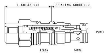
This is a normally closed, balanced poppet, switching element. When the external vent port is blocked, the poppet remains in the closed position. Venting the external port shifts it to the open position, provided there is sufficient pressure at port 3.
