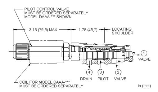
This is a normally closed, balanced poppet, switching element with an integral T-8A control cavity. With a 2-way valve in the closed position installed in the T-8A control cavity, the poppet remains closed. Opening the 2-way valve shifts the poppet to the open position, provided there is sufficient pressure at port 3.
