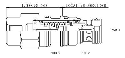
This is a normally closed, balanced poppet, switching element. Pilot pressure at port 3 shifts the valve to the open position.
