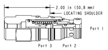
This is a normally closed, balanced poppet, switching element. When the external vent port is blocked, the poppet remains in the closed position. Venting the external port shifts it to the open position, provided there is sufficient pressure at port 3.
