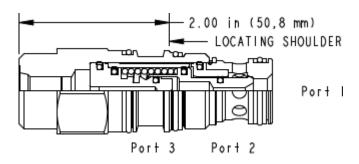
This is a normally closed, balanced poppet, switching element. When the external vent port is blocked, the poppet remains in the closed position. Venting the external port shifts it to the open position, provided there is sufficient pressure at port 3.
