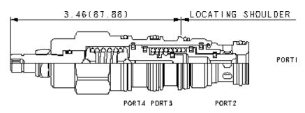
This is a normally closed, balanced poppet, switching element. When pilot pressure is applied to port 3, the poppet remains closed until the pilot pressure reaches the setting established by the integral pilot relief stage, at which point the poppet shifts to the open position.
