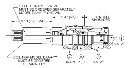
This is a normally closed, balanced poppet, switching element with an integral T-8A control cavity. With a 2-way valve in the closed position installed in the T-8A control cavity, the poppet remains closed. Opening the 2-way valve shifts the poppet to the open position, provided there is sufficient pressure at port 3.
