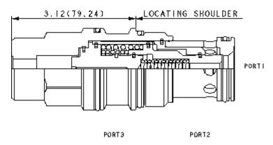
This is a normally closed, balanced poppet, switching element. Pilot pressure at port 3 shifts the valve to the open position.
