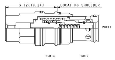
This is a normally closed, balanced poppet, switching element. When the external vent port is blocked, the poppet remains in the closed position. Venting the external port shifts it to the open position, provided there is sufficient pressure at port 3.
