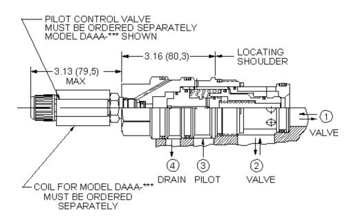
This is a normally closed, balanced poppet, switching element with an integral T-8A control cavity. With a 2-way valve in the closed position installed in the T-8A control cavity, the poppet remains closed. Opening the 2-way valve shifts the poppet to the open position, provided there is sufficient pressure at port 3.
