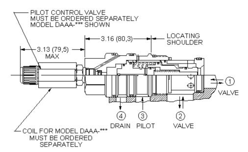
This is a normally closed, balanced poppet, switching element with an integral T-8A control cavity. With a 2-way valve in the closed position installed in the T-8A control cavity, the poppet remains closed. Opening the 2-way valve shifts the poppet to the open position, provided there is sufficient pressure at port 3.
