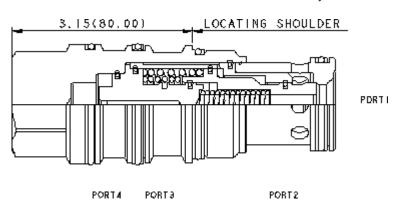
This is a normally closed, balanced poppet, switching element. Pilot pressure at port 3 shifts the valve to the open position.
