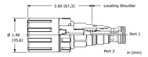
This manually operated, 2-position, 2-way directional cartridge is a direct-acting, balanced spool valve used to control the direction of flow in a hydraulic circuit. The valve is available in either a normally open or normally closed configuration. Manual operation is achieved via Sun's Twist/Lock manual override mechanism and is designed for intermittent (infrequent) use only.
