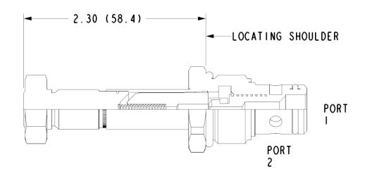
This solenoid-operated, 2-way, 2-position spool valve is a direct-acting, balanced spool directional valve. The valve is only available in the normally closed configuration. This valve is designed to be used with the 780 Series coils.
