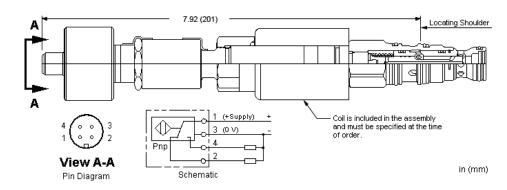
This solenoid-operated 3-way, 2-position cartridge is a direct-
