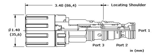
This manually operated, 2-position, 3-way directional cartridge is a direct-acting, balanced spool valve used to control the direction of flow in a hydraulic circuit. Manual operation is achieved via Sun's Twist/Lock manual override mechanism and is designed for intermittent (infrequent) use only.
