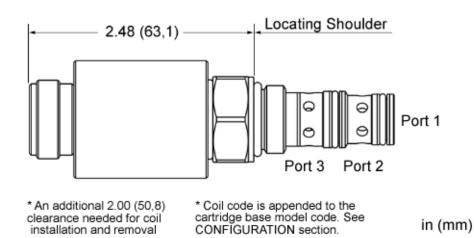
This solenoid-operated 3-way, 2-position cartridge is a direct-acting, balanced spool directional valve.
