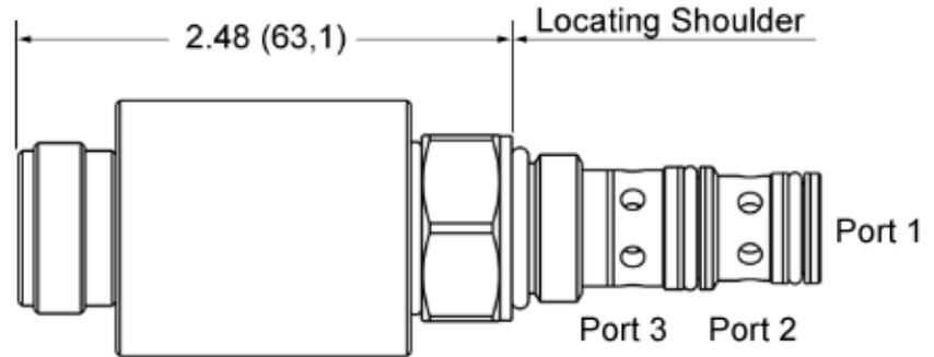
\* An additional 2.00 (50,8) clearance needed for coil installation and removal
