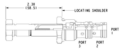
This solenoid-operated 3-way, 2-position cartridge is a direct-acting, balanced spool directional valve. This valve is designed to be used with the 780 Series coils.
