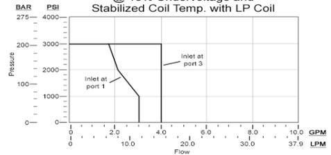
Note: Performance limits are derived with 4-way operation and symmetrical flow. For valve applications where either asymmetrical flow or 3-way operation is present, these performance limits may be reduced.
