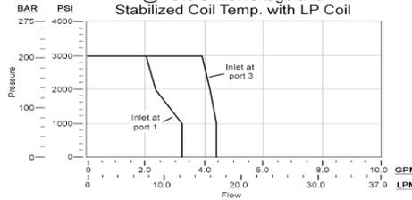
Note: Performance limits are derived with 4-way operation and symmetrical flow. For valve applications where either asymmetrical flow or 3-way operation is present, these performance limits may be reduced.
