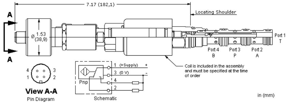
This solenoid-operated, 4-way, 2-position cartridge is a direct-acting, balanced spool directional valve. The transition between positions is closed. The closed transition greatly reduces the loss of oil when shifting which can be of particular importance in pilot control circuits. The position switch provides confirmation that the valve is in the spring biased position. [Click Here for the position sensor pin diagram](https://www.sunhydraulics.com/tech-resources/position-sensor-pin-diagram)
