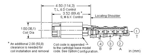
This solenoid-operated 4-way, 2-position cartridge is a direct-acting, balanced spool directional valve with a soft shift feature. The soft shift feature greatly reduces system shock due to valve actuation.
