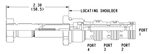
This solenoid-operated 4-way, 2-position cartridge is a direct-acting, balanced spool directional valve. This valve is designed to be used with the 780 Series coils.
