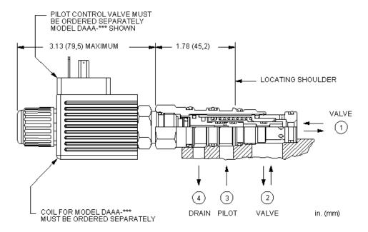
This is a normally open, balanced poppet, switching element with an integral T-8A control cavity. With a 2-way valve in the closed position installed in the T-8A control cavity, the poppet remains open. Opening the 2-way valve shifts the poppet to the closed position, provided there is sufficient pressure at port 3.
