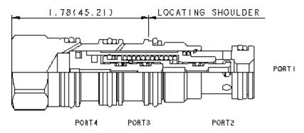
This is a normally open, balanced poppet, switching element. Pilot pressure at port 3 shifts the valve to the closed position.
