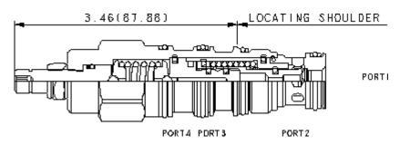
This is a normally open, balanced poppet, switching element. When pilot pressure is applied to port 3, the poppet remains open until the pilot pressure reaches the setting established by the integral pilot relief stage, at which point the poppet shifts to the closed position.
