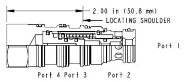
This is a normally open, balanced poppet, switching element. When the vent port (port 4) is blocked, the poppet remains in the open position. Venting port 4 shifts it to the closed position, provided there is sufficient pressure at port 3.
