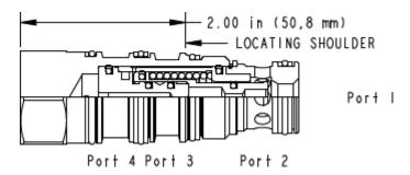
This is a normally open, balanced poppet, switching element. When the vent port (port 4) is blocked, the poppet remains in the open position. Venting port 4 shifts it to the closed position, provided there is sufficient pressure at port 3.
