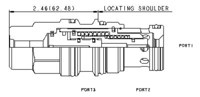
This is a normally open, balanced poppet, switching element. Pilot pressure at port 3 shifts the valve to the closed position.
