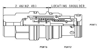
This is a normally open, balanced poppet, switching element. When the external vent port is blocked, the poppet remains in the open position. Venting the external port shifts it to the closed position, provided there is sufficient pressure at port 3.
