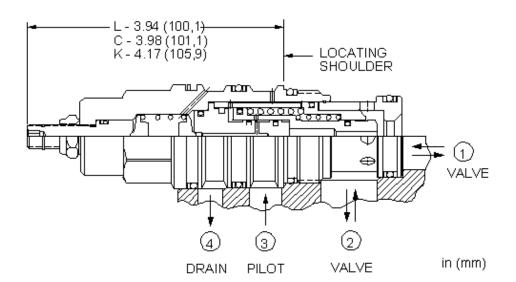
This is a normally open, balanced poppet, switching element. When pilot pressure is applied to port 3, the poppet remains open until the pilot pressure reaches the setting established by the integral pilot relief stage, at which point the poppet shifts to the closed position.
