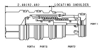
This is a normally open, balanced poppet, switching element. When the vent port (port 4) is blocked, the poppet remains in the open position. Venting port 4 shifts it to the closed position, provided there is sufficient pressure at port 3.
