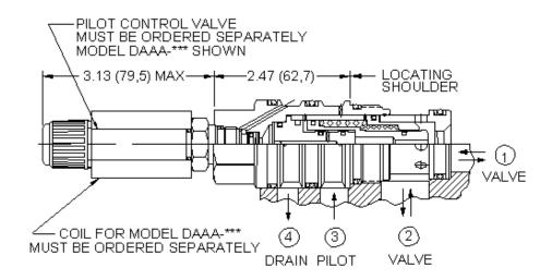
This is a normally open, balanced poppet, switching element with an integral T-8A control cavity. With a 2-way valve in the closed position installed in the T-8A control cavity, the poppet remains open. Opening the 2-way valve shifts the poppet to the closed position, provided there is sufficient pressure at port 3.
