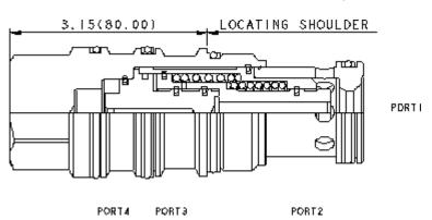
This is a normally open, balanced poppet, switching element. When the vent port (port 4) is blocked, the poppet remains in the open position. Venting port 4 shifts it to the closed position, provided there is sufficient pressure at port 3.
