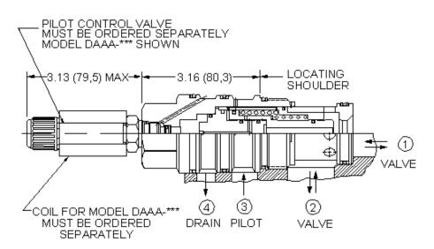
This is a normally open, balanced poppet, switching element with an integral T-8A control cavity. With a 2-way valve in the closed position installed in the T-8A control cavity, the poppet remains open. Opening the 2-way valve shifts the poppet to the closed position, provided there is sufficient pressure at port 3.
