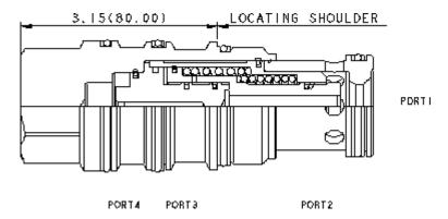
This is a normally open, balanced poppet, switching element. Pilot pressure at port 3 shifts the valve to the closed position.
