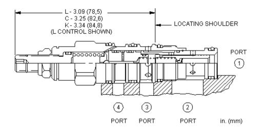
Normally open, pilot-operated, 2-way directional cartridges are switching devices typically used in moderate flow circuits. They can be used by themselves or to actuate larger pilot-operated directional cartridges or logic cartridges. The valve shifts when the pressure differential between port 1 and port 4 exceeds the setting.
