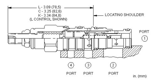
Pilot-operated, 3-way directional cartridges (1 blocked, 2-to-3 open) are switching devices typically used in moderate-flow circuits. They can be used by themselves or to actuate larger pilot-operated directional cartridges or logic cartridges. The valve shifts when the pressure differential between port 1 and port 4 exceeds the setting.
