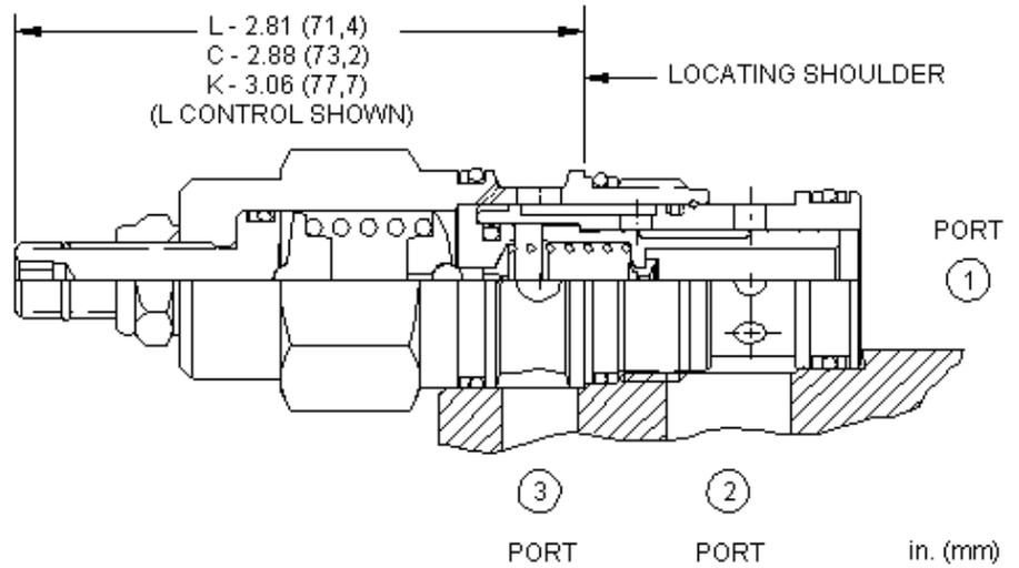
Normally open, pilot-operated, 2-way directional cartridges are switching devices typically used in moderate flow circuits. They can be used by themselves or to actuate larger pilot-operated directional cartridges or logic cartridges. The valve shifts when the pressure differential between port 1 and port 3 exceeds the setting.
