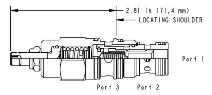
Pilot-operated, 3-way directional cartridges (1 blocked, 2 to 3 open) are switching devices typically used in moderate flow circuits. They can be used by themselves or to actuate larger pilot-operated directional cartridges or logic cartridges. The valve shifts when the pressure differential between port 1 and port 3 exceeds the setting.
