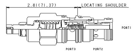
Pilot-operated, 3-way directional cartridges (1 to 2 open, 3 blocked) are switching devices typically used in moderate flow circuits. They can be used by themselves or to actuate larger pilot-operated directional cartridges or logic cartridges. The valve shifts when the pressure differential between port 1 and port 3 exceeds the setting.
