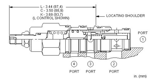
Normally open, pilot-operated, 2-way directional cartridges are switching devices typically used in moderate flow circuits. They can be used by themselves or to actuate larger pilot-operated directional cartridges or logic cartridges. The valve shifts when the pressure differential between port 1 and port 4 exceeds the setting.
