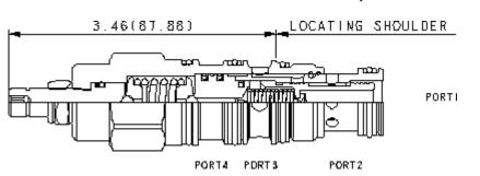
Pilot-operated, 3-way directional cartridges (1 to 2 open, 3 blocked) are switching devices typically used in moderate flow circuits. They can be used by themselves or to actuate larger pilot operated directional cartridges or logic cartridges. The valve shifts when the pressure differential between port 1 and port 4 exceeds the setting.
