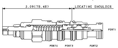
The normally-open, direct-acting 2-way directional cartridge with external drain is a pilot unloading valve used to sense pressure in one circuit to switch or unload a valve in a different circuit. When pressure at port 1 exceeds the setting of the valve, the spool shifts to block port 2 from port 3.
