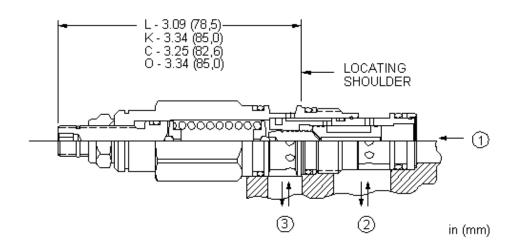
Direct-acting, 3-way directional cartridges (1 blocked, 2 to 3 open) are switching devices typically used in moderate flow circuits. They can be used by themselves or to actuate larger pilot-operated directional cartridges or logic cartridges. The valve shifts when the pressure differential between port 1 and port 3 exceeds the setting.
