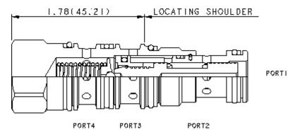
Normally open, direct-acting, 2-way directional cartridges are switching devices typically used in moderate flow circuits. They can be used by themselves or to actuate larger pilot operated directional cartridges or logic cartridges. The valve shifts when the pressure differential between port 1 and port 4 exceeds the setting.
