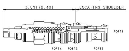
Normally closed, direct-acting, 3-way directional cartridges are switching devices typically used in moderate flow circuits. They can be used by themselves or to actuate larger pilot-operated directional cartridges or logic cartridges. The valve shifts when the pressure differential between port 1 and port 4 exceeds the setting.
